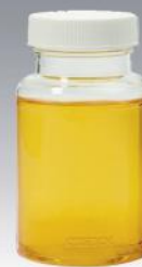
Yellow is positive for total coliforms.
