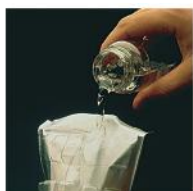
2. POUR SAMPLE/ COLILERT MIXTURE INTO QUANTI-TRAY.
