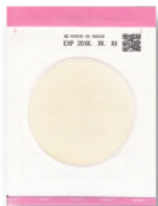
5300-50 Aerobic Bacteria Incubation: 48 ± 2 hours at 35°C ±1°C
