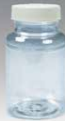
Clear is negative for total coliforms and E. coli .
