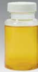
Yellow is positive for total coliforms.
