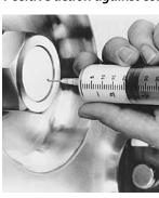
Bacterial and phage contamination can occur in any processing plant ... at any time. Don't take chances. Take action against contamination with the QualiTru Aseptic Transfer System. These aseptic injection ports can be installed in your processing tanks or vats for the aseptic transfer of cultures and viscous materials. A sterile syringe and needle transfers ingredients into
