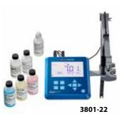
identify when pH meter and ORP meter readings are complete. View active pH, ORP and temperature calibration logs with date and time stamp, record key measurements using the 500-point data log with date and time stamp and output all logs to a printer or computer.
