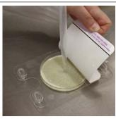
Step 3 • Rapidly dispense 5.0 mL of sample, or sample dilution, onto the center of exposed plate.
