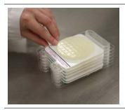
Step 5 • Incubate plates in the dark with clear side up, as shown.
