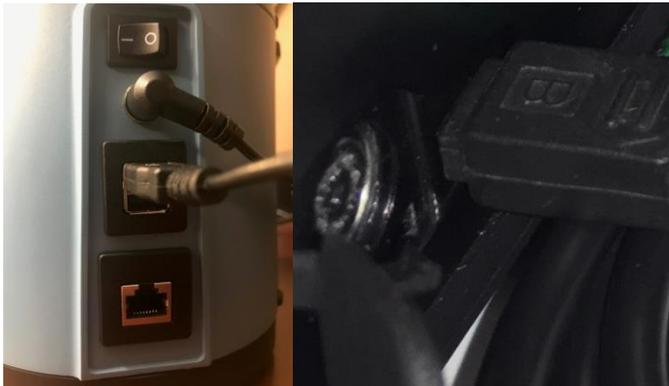
**Figure 40** USP connections on Counter and on Printer
