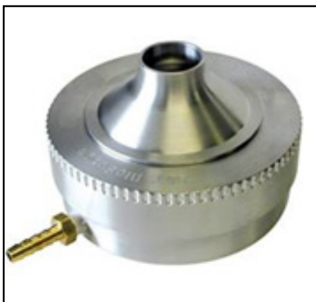
Figure 1. SKC single stage particle sampler. An agar plate sits in the inside of the unit. The device is attached to a calibrated vacuum pump which pulls air through the pin point holes onto the petri dish at a rate of 0.9994 CF/min (28.3 L/min).
